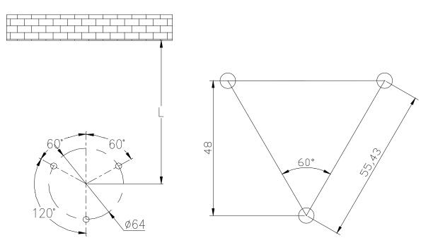
Make sure the Awning is projected. According to the assembly diagram, choose 3 points of the below part of the Awning's front bar.
