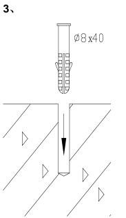
Install plastic expansion tubes into the 3 holes
