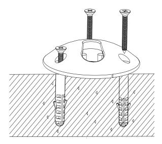
Align the three holes on the outside of the base to the three plastic expansion tubes on the ground and tighten them with three self-tapping screws clockwise.  $5_{s}$
