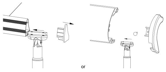
Tighten the screw of the fixed nut plate with the cross screwdriver, then knock back the plastic cover.
